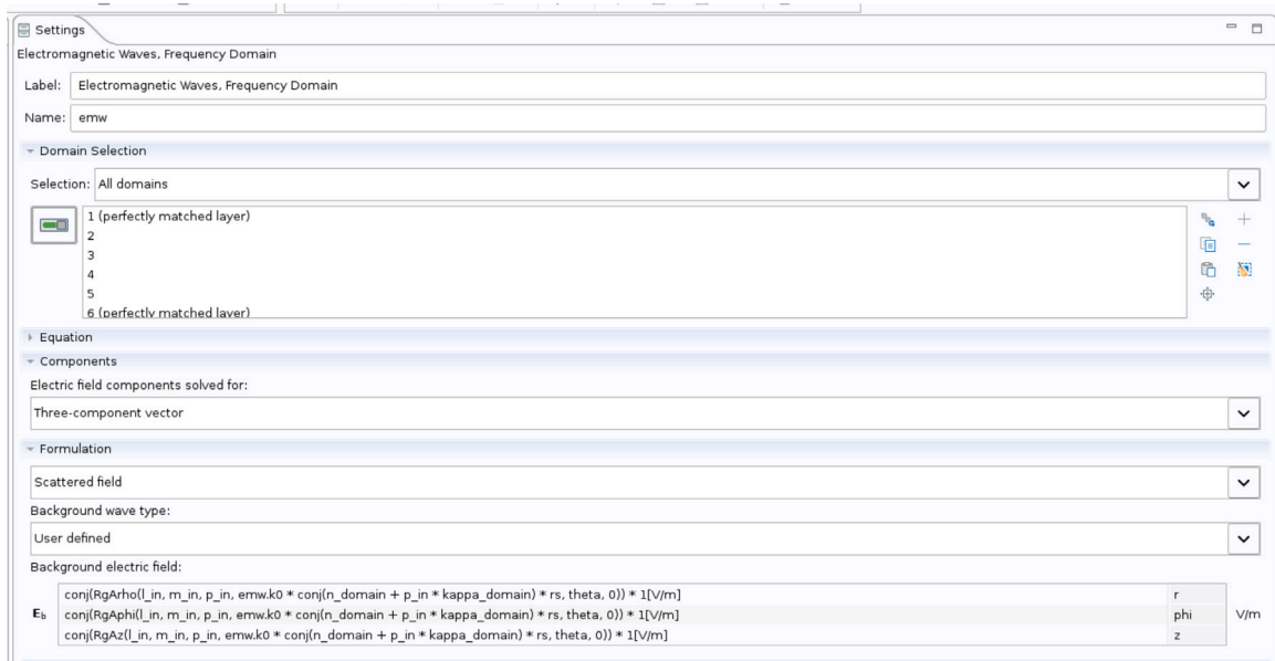
Fig. 3. COMSOL: Background electric field definition in the GUI.
